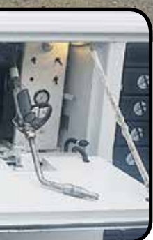
Vanair Air-N-Arc has a remote-control panel mounted at the back of the truck.
