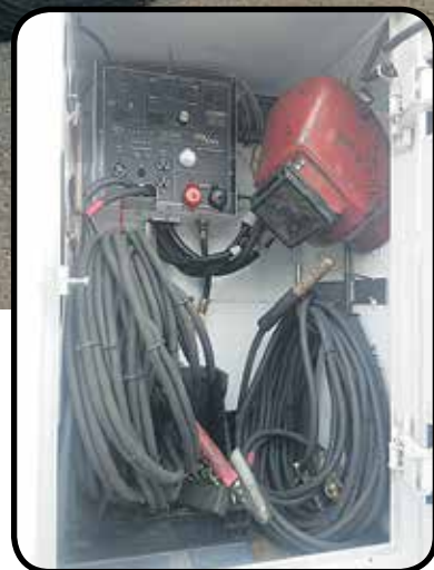
Vanair Air-N-Arc has a remote-control panel mounted at the back of the truck.
